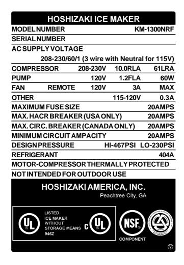
See the Nameplate for electrical and refrigeration specifications. This Nameplate is located on the upper right hand side of rear panel.
